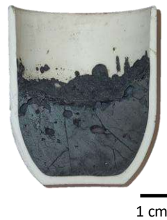
Figure 1: crucible cut in half after a test with 10% alumina, 10°C/h cooling
