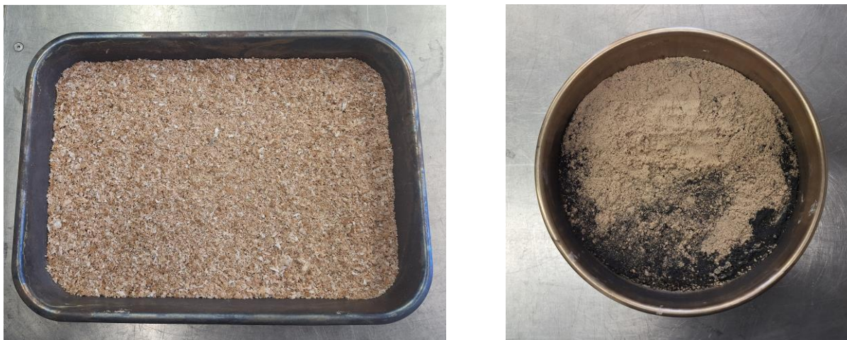
Figure 2: Spruce wood ash, left: ashed >500 \mu\text{m} fraction; right: partially ashed < 80 \mu\text{m} fraction
