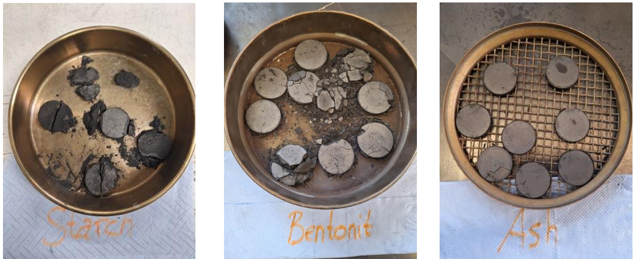
Figure 4: Biochar briquettes after curing time; left to right: starch bound bentonite-bound, ash-bound
