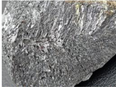
Figure 4: The obtained crystalline structure of tin sulfide
