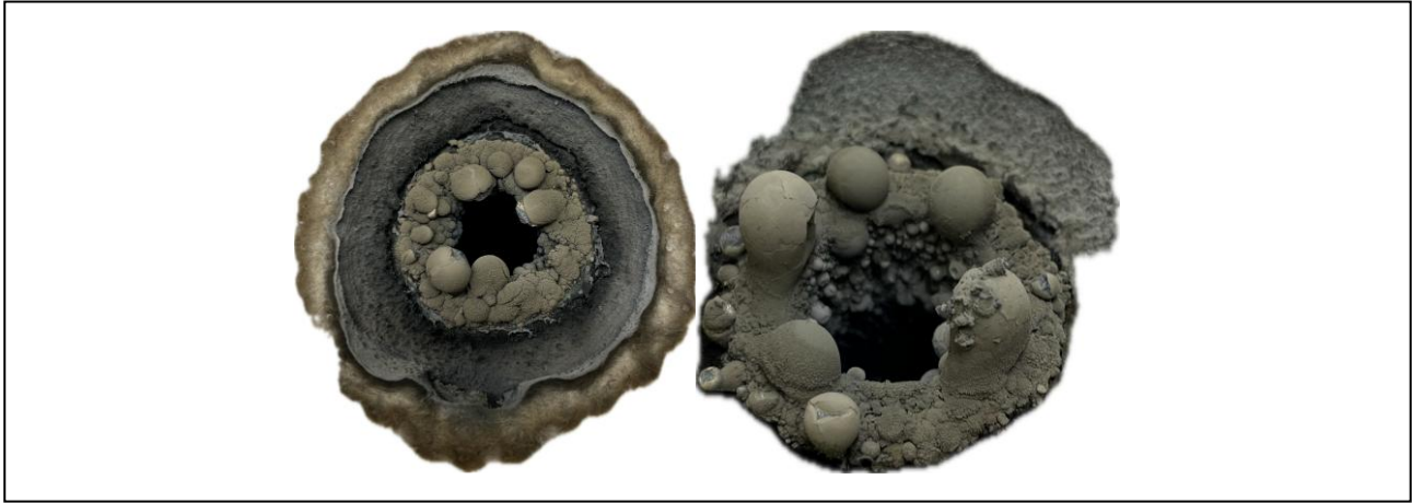
Figure 5: Photos of the distillate found at the bottom of the riser tube from selected experiments. Riser tube diameter is 2.5 cm.
