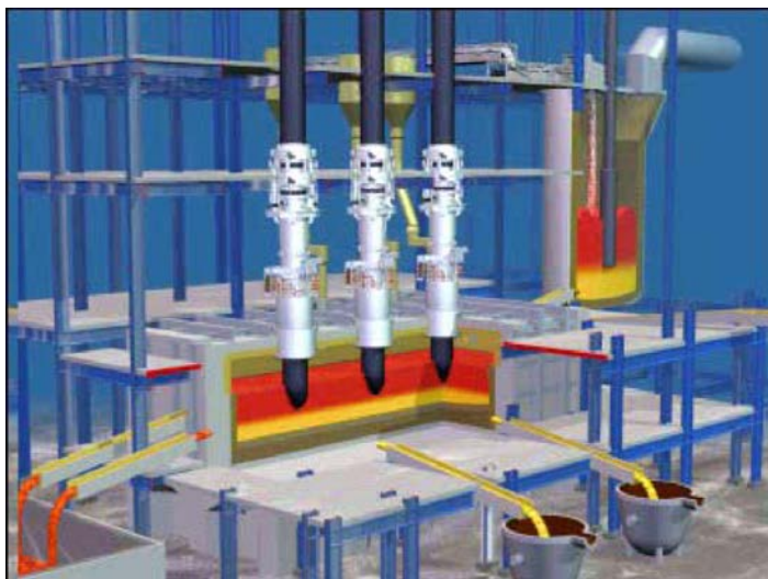
Figure 4: 3D illustration of a rectangular slag cleaning furnace [5]
