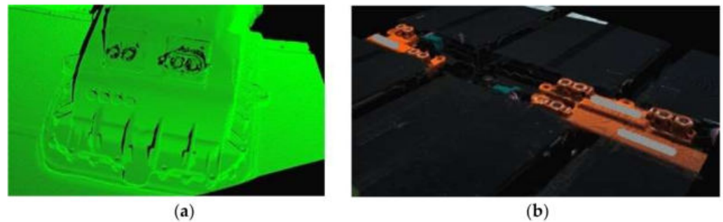
Figure 8. Point cloud of the switch box (a), modules and busbars (b) that were captured with Zivid Two.
