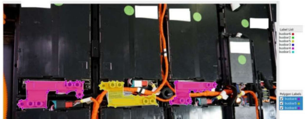
Figure 9. Annotation for instance segmentation with Labelme with the example of the busbars.
