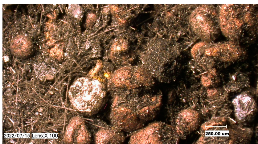
Figure 4. Optical microscopy image of the pyrolyzed and crushed RAM (<0.75 mm) at 100× magnification.
