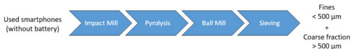
Figure 1. Process chain for the production of a gallium-rich fraction from used smartphones [4].
