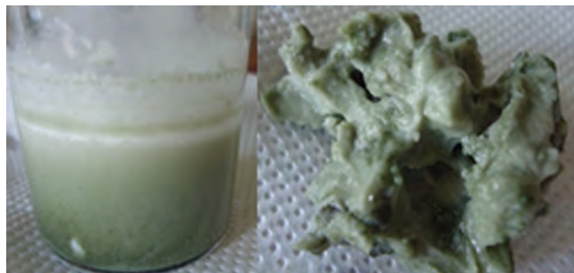
Fig. 3. Gel formation during direct leaching of middlings concentrate with 2M H 2 SO 4 .
