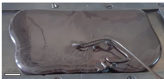
FIGURE 1 Material from conventional melting of red mud containing waste mixture and cooling on steel plate
