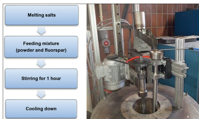
Fig. 3: Steps in the process (left) and arrangement of the experiment in the furnace (right)
