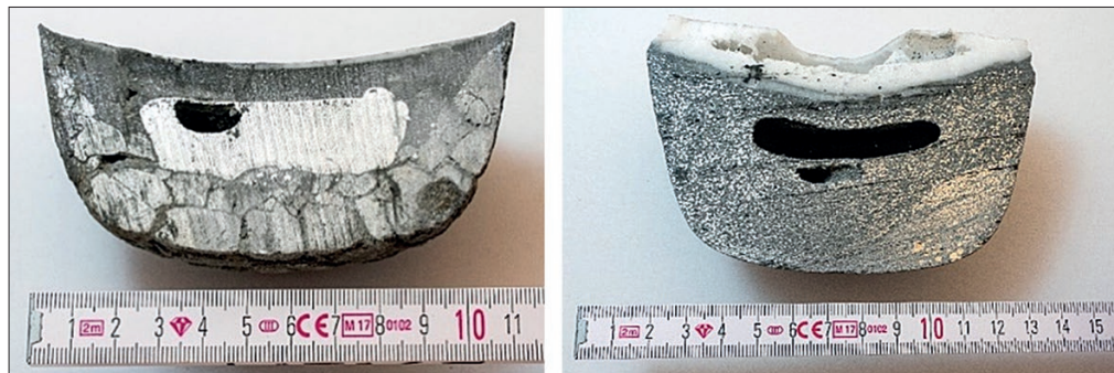
Fig. 5: Adhered powder on the crucible wall
