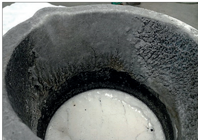
Fig. 5: Adhered powder on the crucible wall
