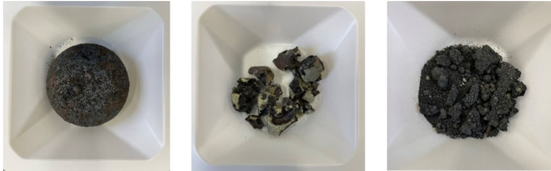
Fig. 4 Exemplary pictures of left: metal; middle: slag; right: powder with metal droplets
