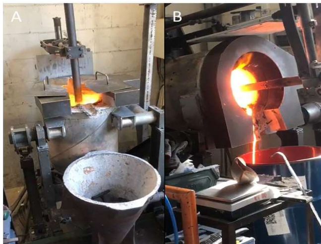
Figure 1A. Smelting of the BR mix with the EAF and Figure 1B. Quenching of the slag in water.
