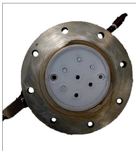
Fig. 1: Lid of the electrolysis cell with white powdery condensate
