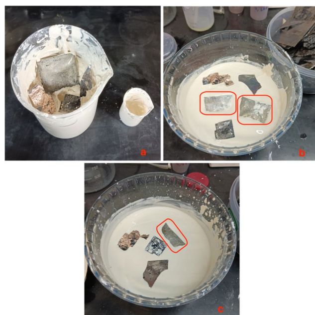
Fig. 6 Pasty material of white-clay with density 1.8 \text{ g}\cdot\text{cm}^{-3} and viscosity 35.7 \text{ g}/(\text{cm}\cdot\text{s}) (a). Suspension of viscosity 0.98 \text{ g}/(\text{cm}\cdot\text{s}) and density 1.34 \text{ g}\cdot\text{cm}^{-3} with batteries into red squares (b). Suspension of viscosity 0.2 \text{ g}/(\text{cm}\cdot\text{s}) and density 1.28 \text{ g}\cdot\text{cm}^{-3} with a battery into a red square (c)
