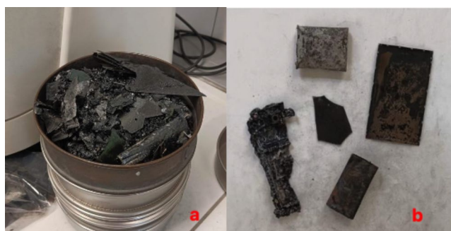
Fig. 2 Mobile phone components after pyrolysis (a) and coarse fraction after 2 cm sieving (b)
