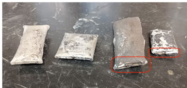
Fig. 1 Batteries from pyrolysis process, in which the two of the left (highlighted in red) are fractured
