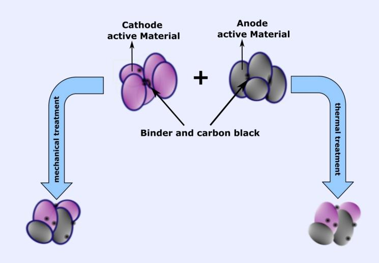
Consequently to pyrolyze or not pyrolyze batteries has a huge impact for the following hydrometallurgy processes.
