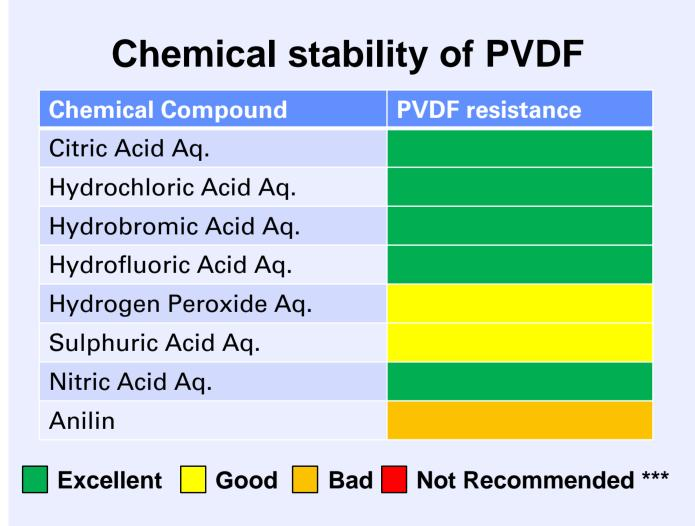
**PVDF** is created as a quite stable Polymer. **Especially against** inorganic chemicals like mineral acids. Additional aging effects not influence the stability significant. The combustion
