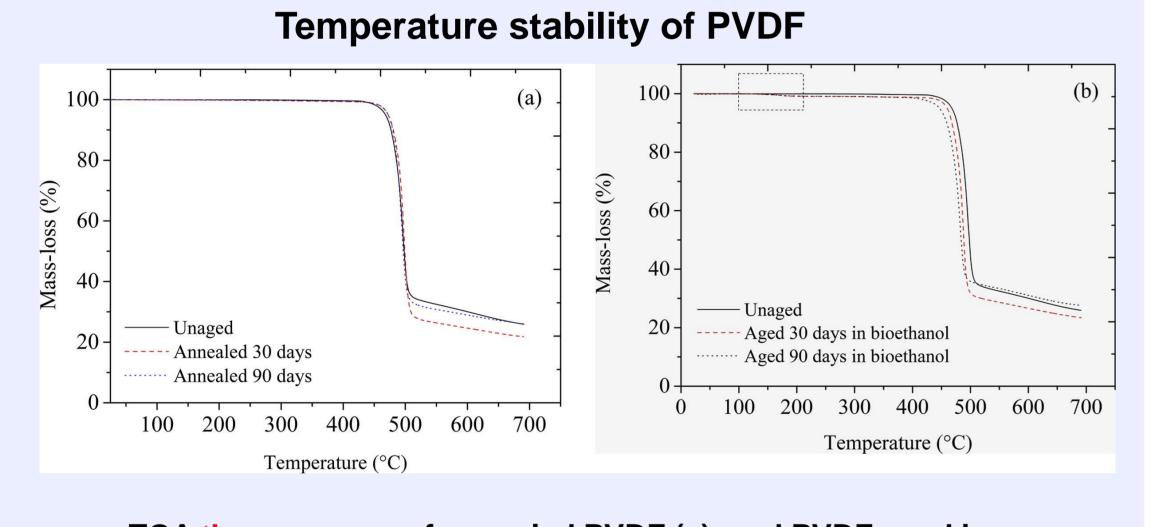
TGA thermograms of annealed PVDF (a), and PVDF aged in bioethanol during experimental times of 30 and 90 days (b), at 20 °C min<sup>-1</sup> heating rate, compared to unaged material.\*\*
