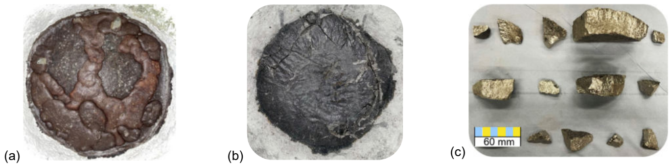
Figure 8: (a) Slag surface, (b) metal surface and (c) metal product of AlCrMoTiV.
