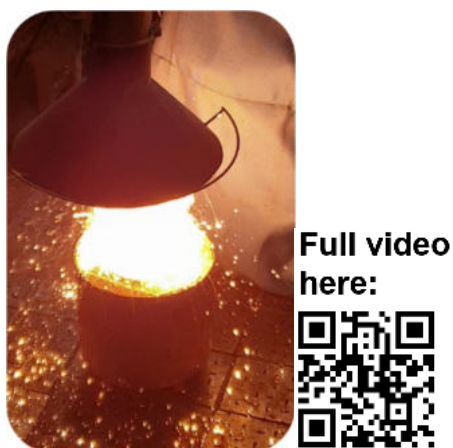
Figure 6: Illustration of the aluminothermic reduction of AlCrMoTiV.
