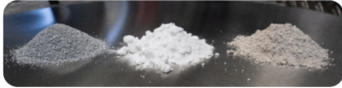
Figure 5: Input materials for ATR process from left to right: Al as reductant, KClO 4 as booster and CaO as flux.
