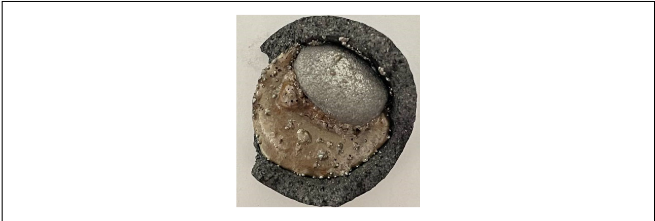
Figure 6: Phases form from carbothermic reduction, silver-grey: metallic phase; brownish-green: MREO phase
