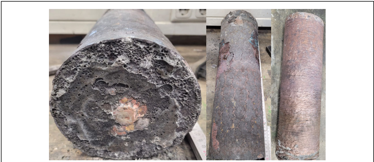
Figure 4: Remelted Ingot, left: bottom side, middle: with slag skin, right: without slag
