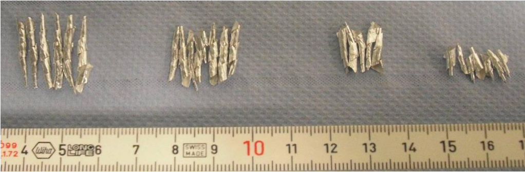
Figure 11: Different chipping sizes distributed in magnesium chippings
