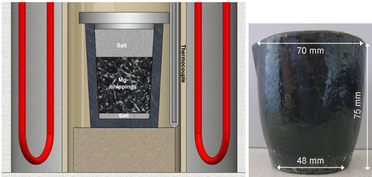
Figure 10: (left) schematic graphite crucible inside the furnace containing Mg-chippings surrounded by two layers of salt mixture and (right) the alumina crucible used for coalescence trials
