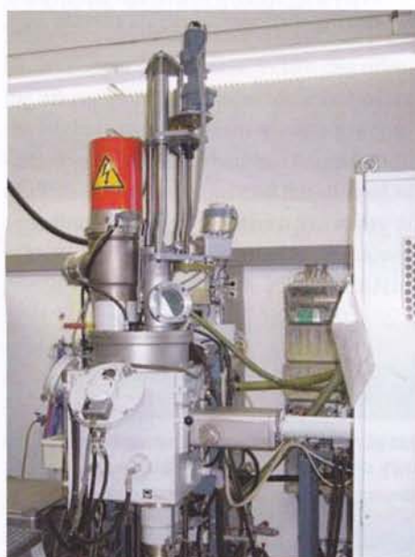
Fig. 15: Electron beam furnace with water cooled copper mould
