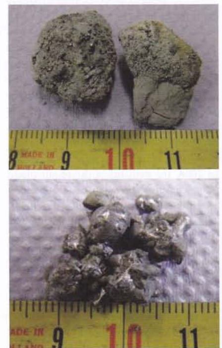
Fig. 6: Melting behaviour of Si-concentrate: top 30 % SiC containing material, bottom 10% SiC containing material
