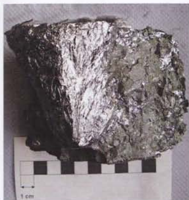
Fig. 7: Result of the melting trial with standard Si-concentrate with (left) and without (right) addition of SiO 2 -CaO slag (ratio CaO/SiO 2 = 1/2)
