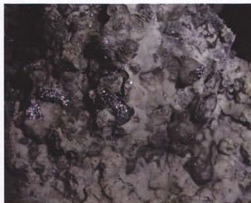
Fig. 7: Result of the melting trial with standard Si-concentrate with (left) and without (right) addition of SiO 2 -CaO slag (ratio CaO/SiO 2 = 1/2)
