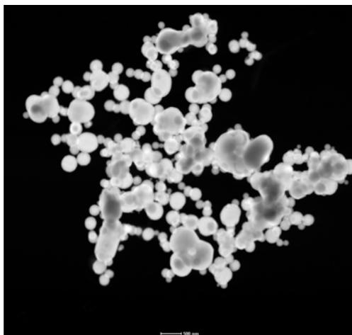
Fig. 5. TEM analysis of USP particles in Exp. 5 (900°C, 0.1 mol/l)
