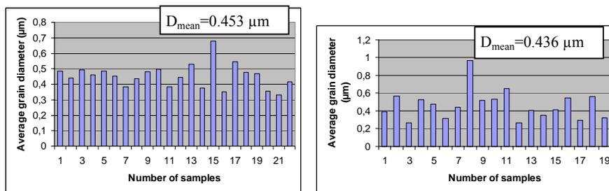
Fig. 9: Mean diameters from particles; left Exp. 1 ( $T=800^{\circ}\text{C}$ ,  $c=0.3\text{ mol/l}$ ), right Exp. 4 ( $T=900^{\circ}\text{C}$ ,  $c=0.3\text{ mol/l}$ )
