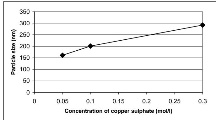
Fig. 7. Calculated solid particle size after USP dependent on the precursor concentration
