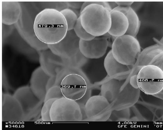
Fig. 3c: Cu particles produced at 900°C, 0.3 mol/l, Exp. 4
