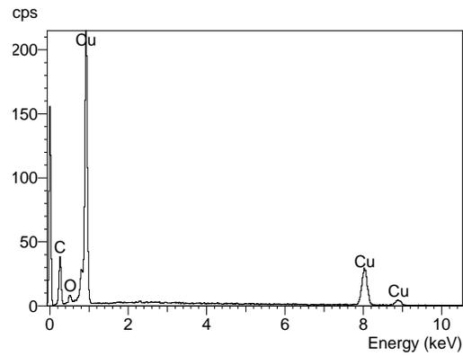
Fig. 4d: EDS analysis of Cu particles produced at 900°C, Exp. 6
