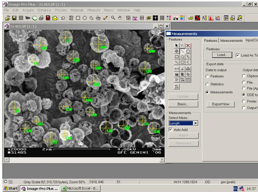
Fig. 8. Image analysis of SEM results for particle size measurement (Exp. 1)
