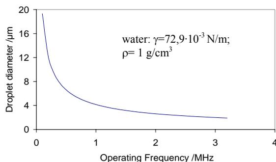
Fig. 6: Calculated aerosol droplet size dependent on the ultrasonic frequency
