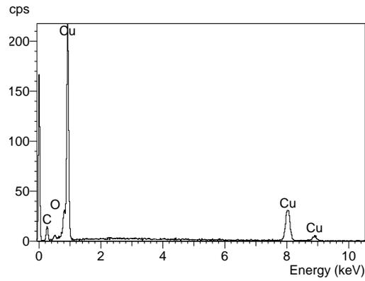
Fig. 4b: EDS analysis of Cu particles produced at 900°C, Exp. 5
