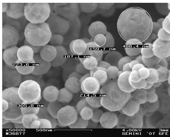
Fig. 4a: Cu particles produced at 900°C, 0.1 mol/l, Exp. 5
