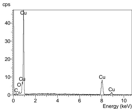
Fig. 3d: EDS analysis of Cu particles produced at 900°C, Exp. 4
