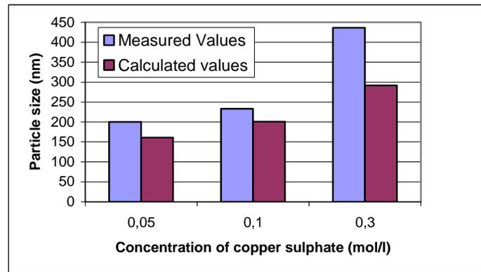
Fig. 11. Experimental and theoretical diameters of particles of copper obtained at  $900^{\circ}\text{C}$  with 2.5 MHz ultrasound frequency and three precursor concentrations
