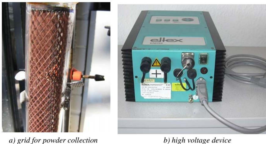
Fig. 2. ESP-system for collection of nanosized powder
