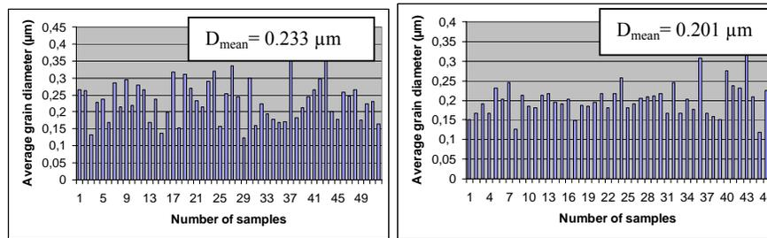
Fig. 10: Mean diameters from particles; left Exp. 5 ( $T=900^{\circ}\text{C}$ ,  $c=0.1 \text{ mol/l}$ ), right Exp. 6 ( $T=900^{\circ}\text{C}$ ,  $c=0.05 \text{ mol/l}$ )
