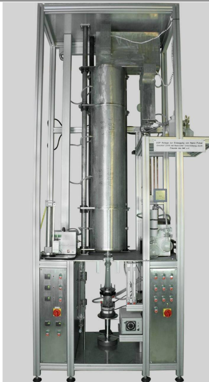
*Fig. 1: Experimental apparatus for the USP-synthesis of copper particles at IME, Aachen*
