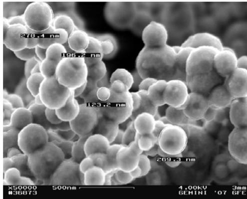
Fig. 4c: Cu particles produced at 900°C, 0.05 mol/l, Exp. 6
