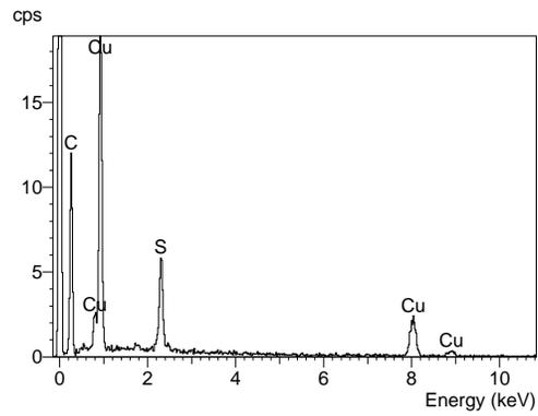
Fig. 3b: EDS analysis of Cu particles produced at 800°C, Exp. 1
