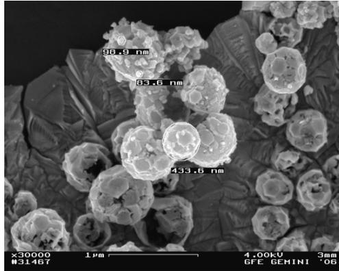
Fig. 3a: Cu particles produced at 800°C, 0.3 mol/l, Exp. 1
