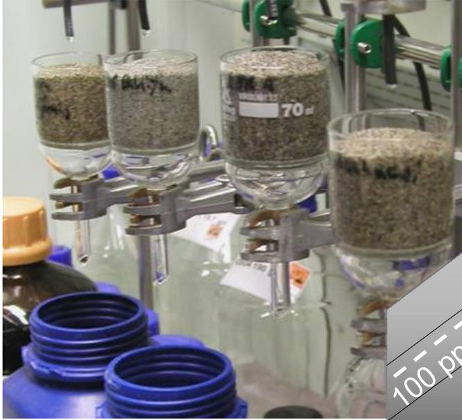
Measuring the adsorption rate by miniature column test.
