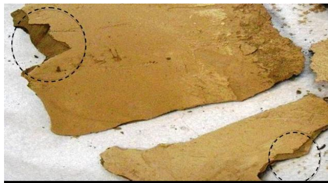
Figure 10: Condensate layers obtained after final distillation at 1200^\circ\text{C}
