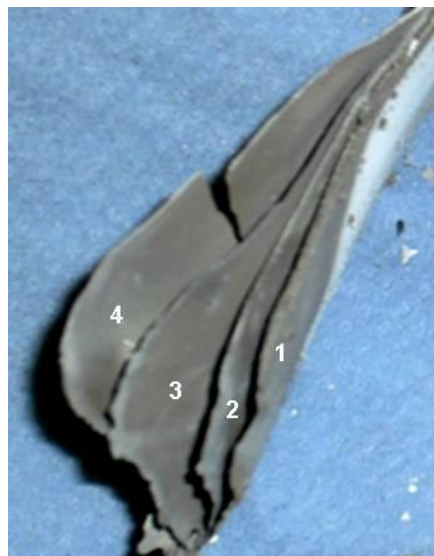
Figure 8: Four layers obtained as condensate material in the quartz tube of a selective distillation at 750°C
