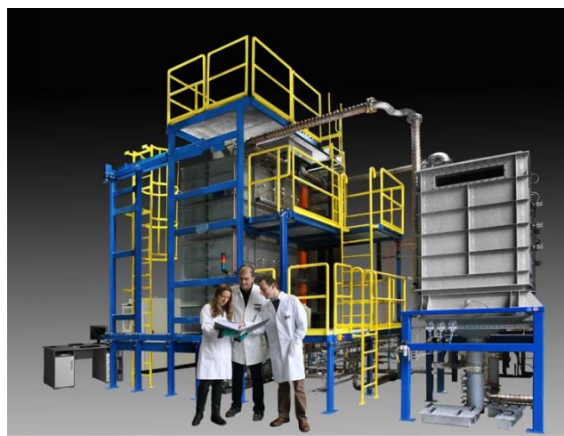
Figure 1: The concept of demo scale USP: 1-Aerosol ultrasonic generator, 2-High-temperature furnace with five wall heated reactors, 3-Electrostatic filter, 4-Vacuum system (left) and photo of the equipment (right) [6]
