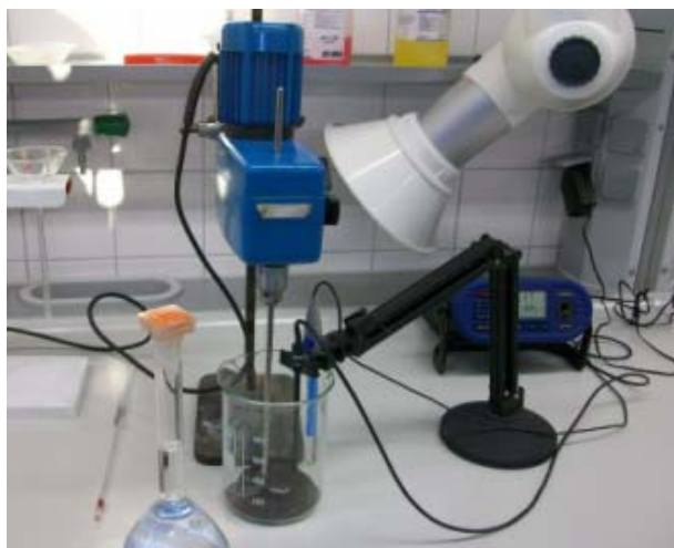
Figure 10. Experimental setup employed for laboratory scale leaching
