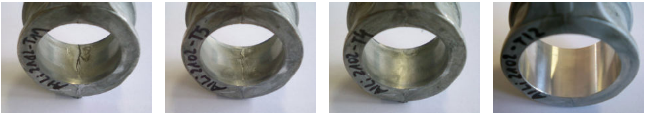
Fig. 6: Hot tearing at the big bearing point: From left to right: a decreasing steel core temperature results in a decreasing hot tear tendency
