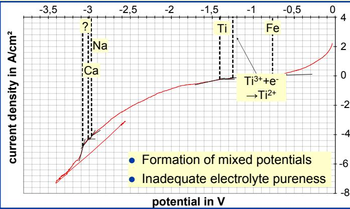
Experimental proof that  $\text{TiCl}_2$  is electrochemically reduced before other electrolyte components
