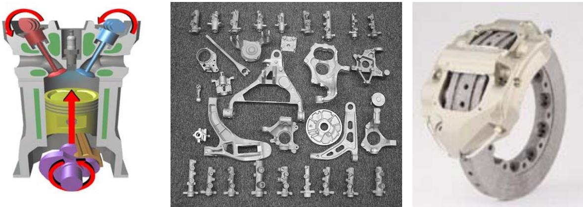
**Fig. 9** : SSM Al-Li future application in high performance engine (left), as substitution for typical automotive casting (middle) and race caliper (right)
