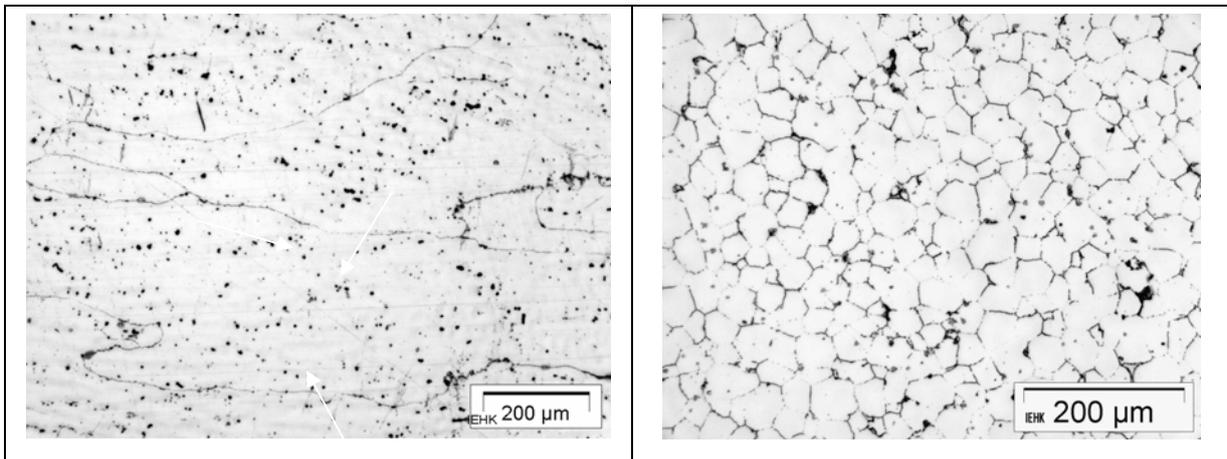
**Fig. 5 :** Effect of Sc,Zr addition on grain size and microstructure of AlLi<sub>2,1</sub>Mg<sub>5,5</sub>Sc<sub>x</sub>Zr<sub>y</sub> (billet N1 0%Sc and 0%Zr left, billet N17 0,15%Sc and 0,15%Zr right)
