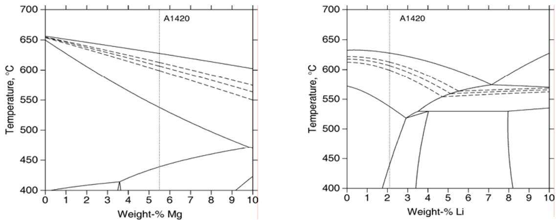
Fig. 1: Calculated isoplethal section at 2,1 weight-% Li (left) and 5,5 weight-% Mg (right)
