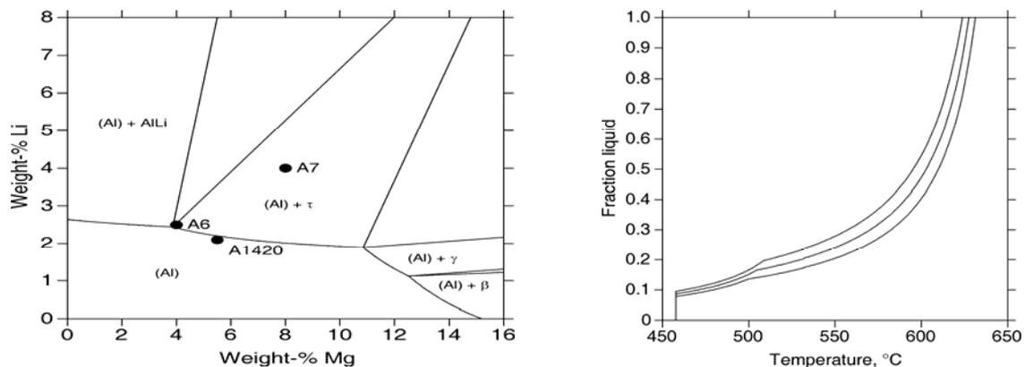
Fig. 2: Calculated isothermal section at 450°C in the Al-Li-Mg system (left) and calculated solidification curves for AlLi<sub>2,1</sub>Mg<sub>5,5</sub> using Scheil-Gulliver approximation (right)
