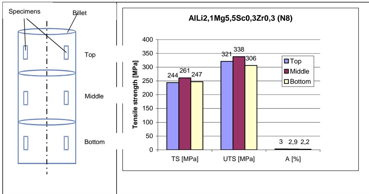
**Fig. 8** : Mechanical properties of synthesized AlLi<sub>2,1</sub>Mg<sub>5,5</sub>Sc<sub>0,3</sub>Zr<sub>0,3</sub> (billet N8) in the as cast condition
