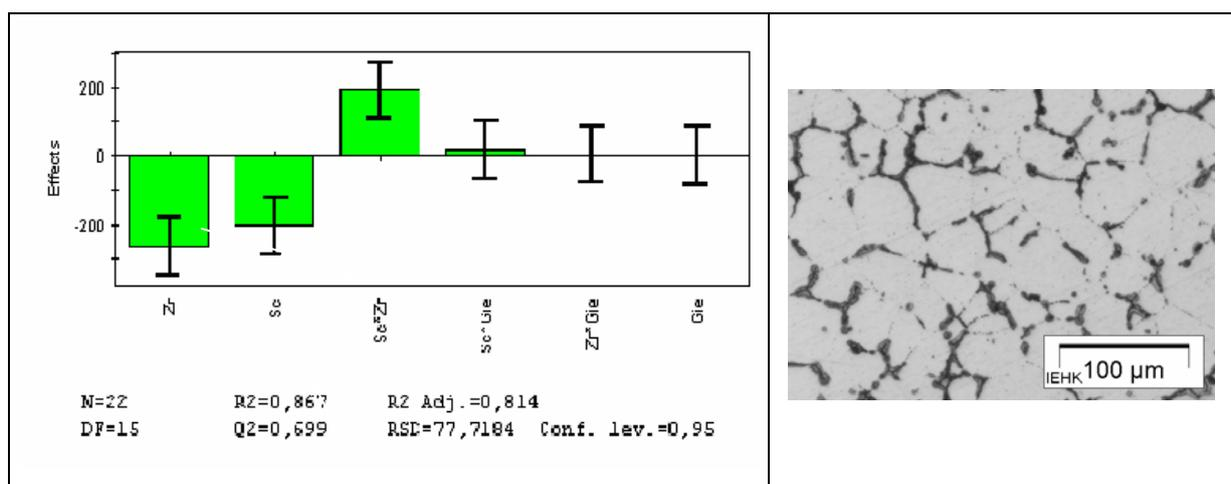
**Fig. 6 :** Statistical effects of Sc and Zr addition (single and mix) and casting temperature (Gie) on grain size of AlLi<sub>2,1</sub>Mg<sub>5,5</sub>ScZr (left), microstructure of billet N17 (right)
