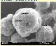
Metal catalysts e.g. Me (Ag, Cu, Co) / ZnO/  $Al_2O_3$  are industrially employed for methanol synthesis and the water gas shift reaction. The strong increase in catalytic activity is a consequence of the resulting higher metal surface area if nanoparticles are used.
