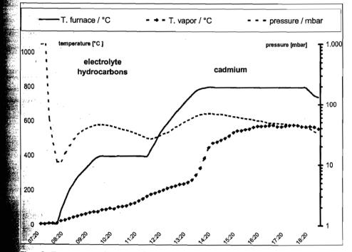
Figure 3: Temperature and Pressure while Treatment of spent NiCad-Batteries
