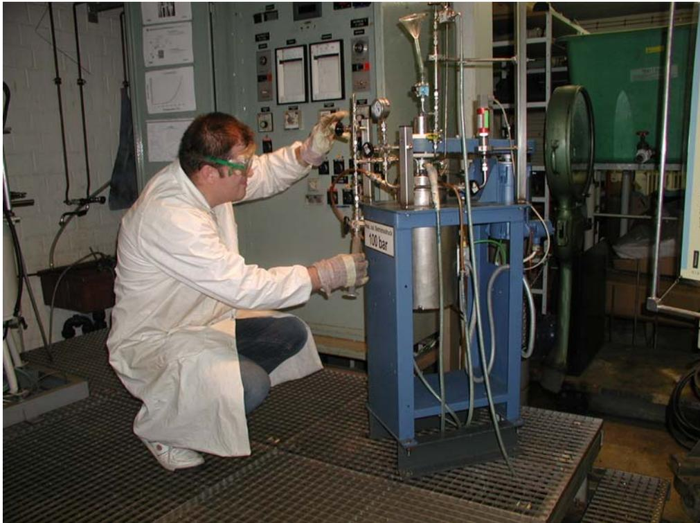
Fig. 1. Sampling at the 2 l –Ti- autoclave at IME, RWTH Aachen [8].
