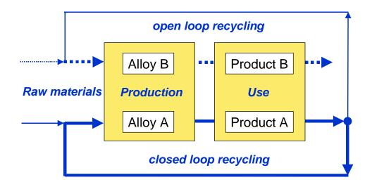
Figure 5: Open and closed recycling cycles
