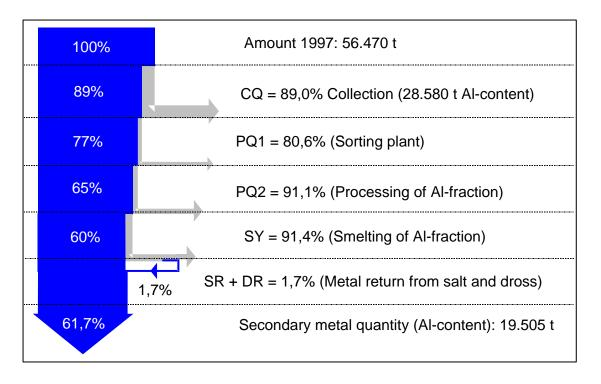
Figure 8: Determination of the recycling quotas for Aluminium light packaging material [6]
