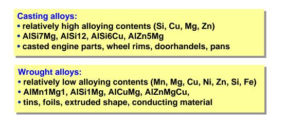
Figure 2: Comparison of casting and wrought alloys
