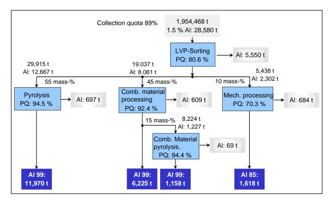
Figure 16: Processing of the Al-fraction of light packaging material [10]
