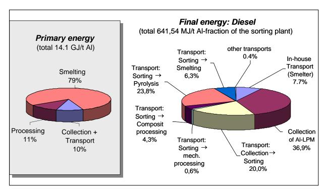
Figure 18: Classification of the primary and final energy consumption for the packaging recycling by the example of Diesel fuel [10]
