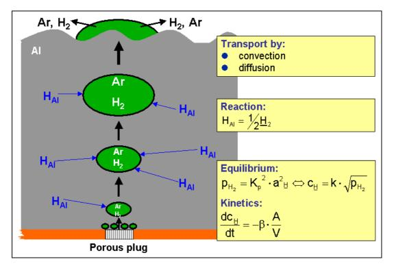
Figure 6: Principle of gas purging
