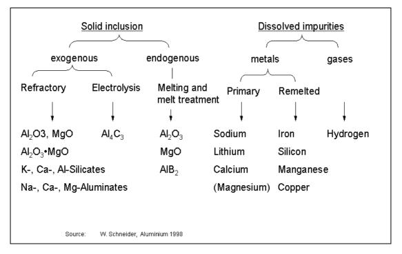
Figure 2: Impurities in aluminium melts
