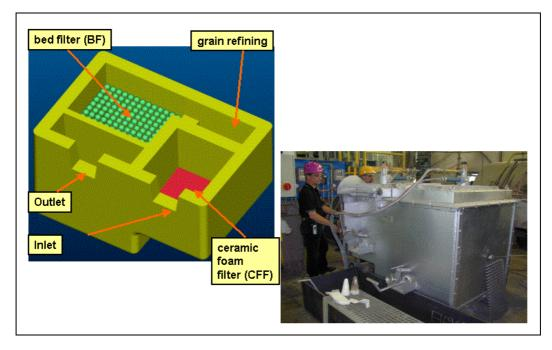
Figure 14: In line aluminium melt treatment: Hydro (VAW)-Filter
