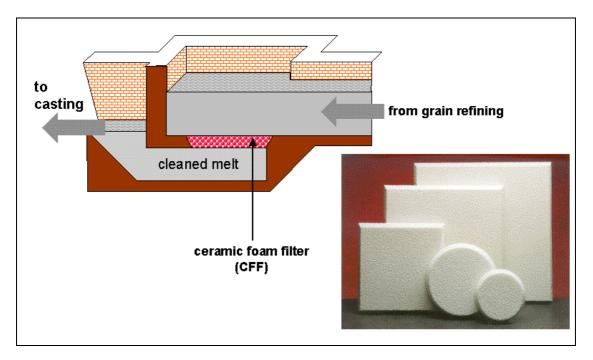
Figure 13: Technology of aluminium melt filtration
