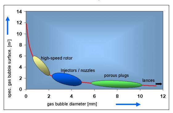
Figure 7: Gas bubble surface versus bubble diameter
