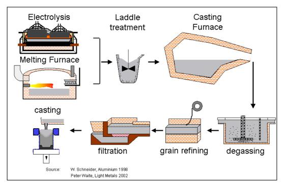
Figure 5: Processing of molten aluminium
