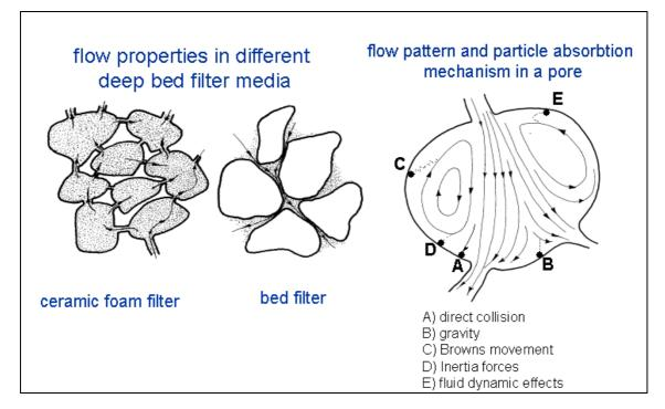
Figure 11: Principles of melt filtration
