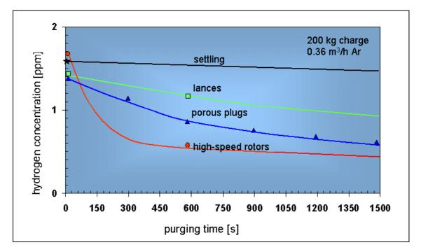
Figure 8: Efficiency of gas purging methods
