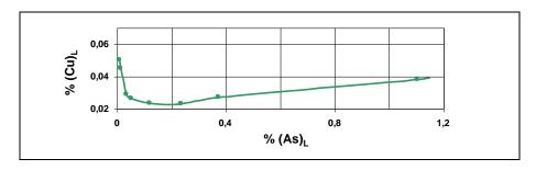
Figure 6: Pb-Cu-As-system; isotherm of Cu-solubility at 337 °C
