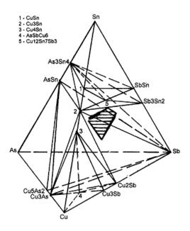
Figure 10: Tetraerdration of the system Cu-Sb-As-Sn
