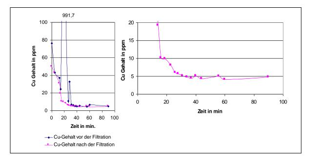
Figure 17: Copper concentration versus reactiontime a) before and after filtration b) detail after filtering
