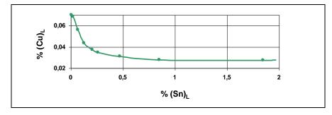
Figure 5: Pb-Cu-Sn-system; isotherm of Cu-solubility at 337 °C
