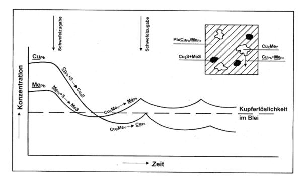
Figure 20: Schematic illustration of proposal mechanism for copper removal
