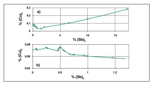
Figure 7: System Pb-Cu-Sb isothermal solubility of copper at 337 °C
