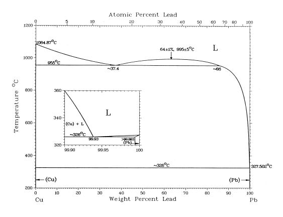
Figure 2: Binary-system Pb-Cu
