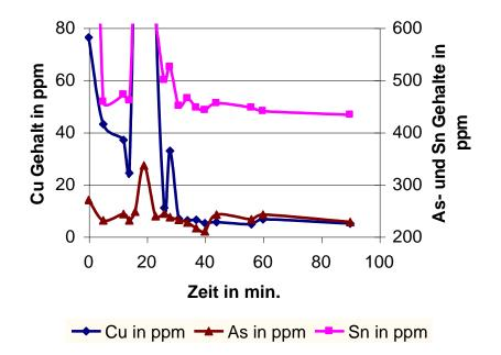
Figure 16: Kinetic curves of copper, tin and arsenic concentration by copper removal in lead with sulphur and pyrite (production samples)
