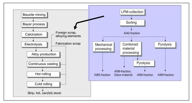
Figure 2: Production and recycling of packaging material
