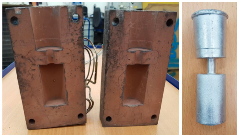
Figure 1. “Sand Hourglass” mold (left) and sample (right).
