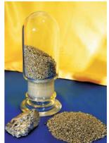
Powders based on hydride forming metals can be produced by using the hydrogenation-dehydrogenation method (HDH). Hydrogenation is an exothermic process by absorbing hydrogen. The product phase is a very brittle hydride, which is subsequently crushed. Dehydrogenation is an endothermic reaction and takes place under vacuum conditions and elevated temperature. The powder is nearly oxygen-free, sinter active and usually shows sizes of 50-150 µm.
