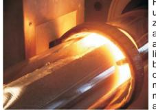
For the production of ultra pure materials zone refining can be applied. A small zone of a metal bar becomes liquid in a tube furnance by a moving induction coil. The liquid zone migrates through the metal bar very slowly and a front of impurities
