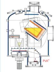
In addition to the conventional casting into steel, water-cooled copper or ceramic moulds, VIM-melts can be poured on a water-cooled rotating disc to form flakes for further powder synthesis using the HDH method. VIM-melts can likewise be treated by moving the rotating crucible downwards through an indirect water-cooling section to constitute directional solidification.
