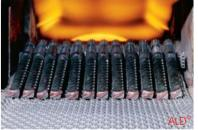
decarbonising or nitration takes place during the heat treatment. Applications are found in processing e.g. titanium or nickel alloys.
