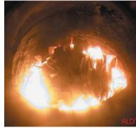
Complex alloys with a maximum batch size of 200 kg are synthesised by using VIM, ESR, VAR or EBM. The intelligent combination of those technologies, the knowledge of suitable VIM-crucibles and raw materials, as well the know-how of process control is the basis for a successful small-scale production of high-tech
